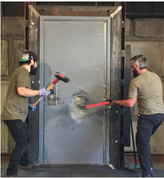
Image from actual forced entry testing
